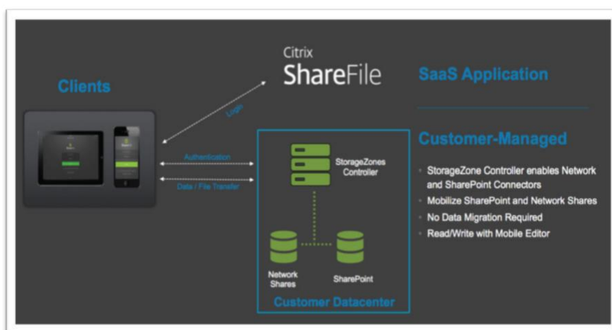
10 11 12 13 14 15 16 17 Figure 3. StorageZone Connector architecture
