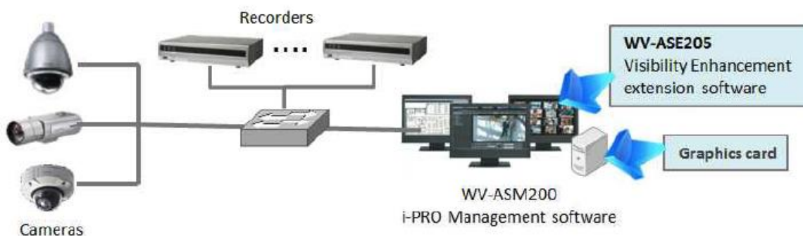
Figure 3: System configuration example of Panasonic Visibility Enhancement Software.
