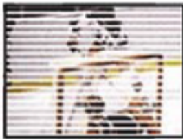
Interlace scanning first scans the odd-numbered lines in 1/60th of a second...
