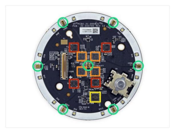
42. Upon information and belief, the Amazon Echo products include a digital signal processor, such as digital signal processors ("DSP"), manufactured by third parties including Texas Instruments, MediaTek, and AMLogic.
