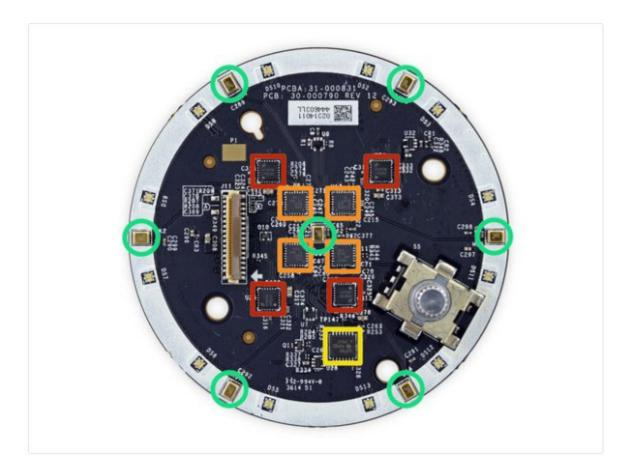
34. Upon information and belief, the Amazon Echo products include a digital signal processor, such as digital signal processors ("DSP"), manufactured by third parties including Texas Instruments, MediaTek, and AMLogic.
